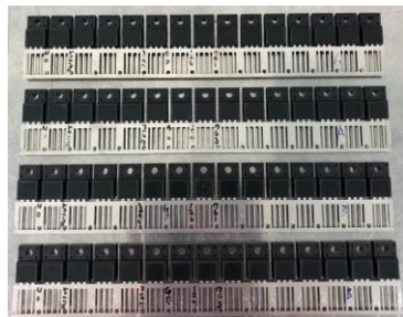
Transfer Molding EMC by 1.) KCC 3097GX 2.) KCC 3097GE
